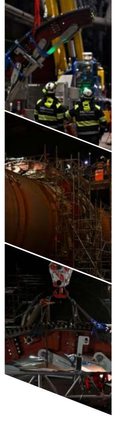
RECOGNISING THE LIMITATIONS OF CONVENTIONAL GIRTH GEARS, DBSANTASALO HAS PIONEERED THE USE OF ADI FOR SEGMENTED GIRTH GEARS.
